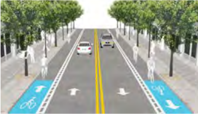
Figure 19. Uni-directional marked cycle lane.
