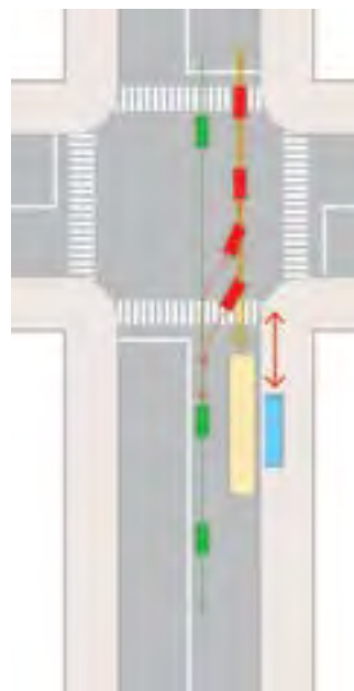
Figure 41. Impact on traffic due to stop positioned close to intersection
