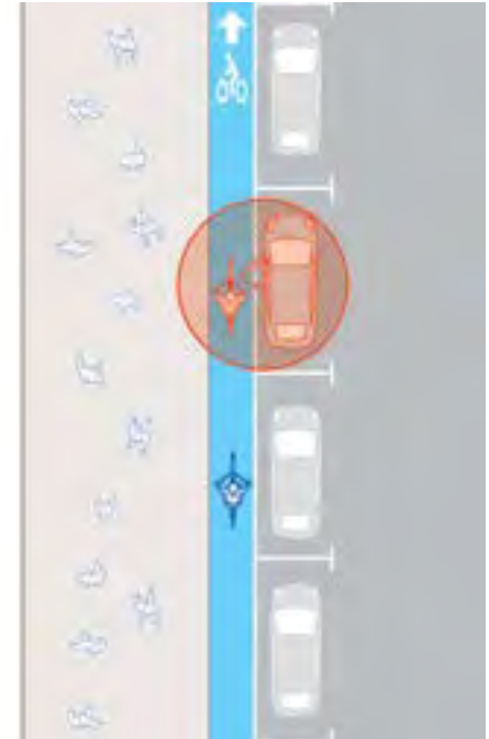
Figure 25. Cycle lane between sidewalk and parking lane without any buffer
