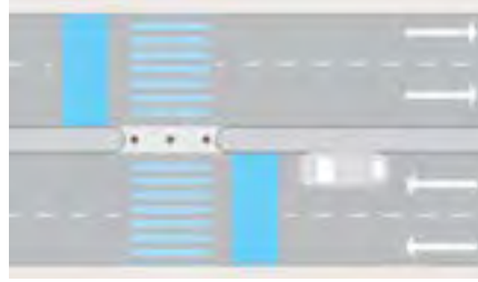
Figure 53. Speed humps before pedestrian crossing.
