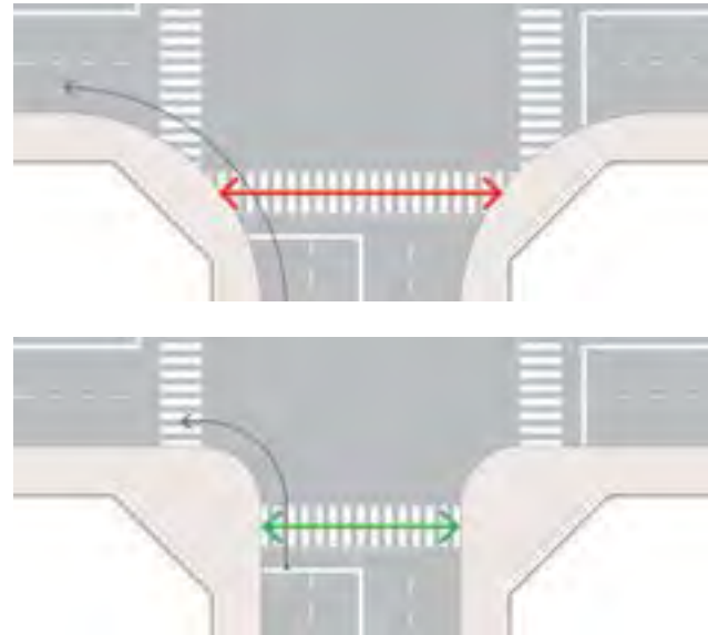
Figure 15. Reduced intersection corner curvature for pedestrian safety Reducing intersection corner curvature increases pedestrian safety as it enables drivers to turn at significantly slower speeds and also reduce pedestrian crossing time.
