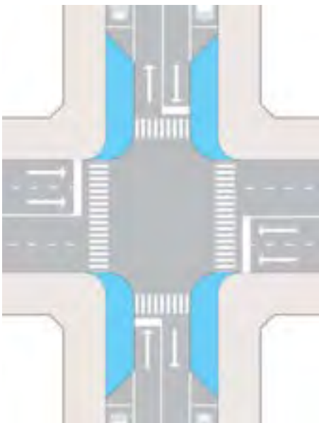
Figure 61. Extending curb corners at intersections to create gateways
