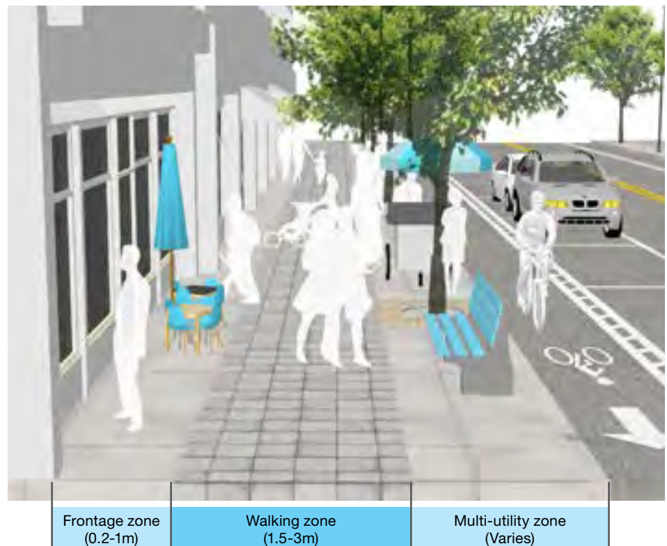
Figure 8. Three components of a sidewalk
