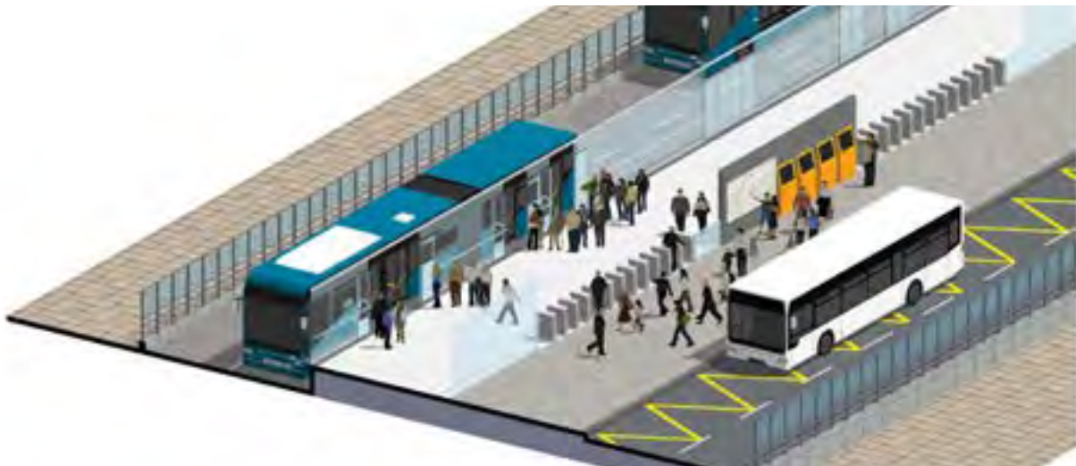
Figure 71. Typical transfer platform at station along Bogota, Colombia's TransMilenio BRT corridor with height differences on either side to accommodate the different floor heights of BRT bus (on left side) and feeder services (right side) (Source: WRI)
