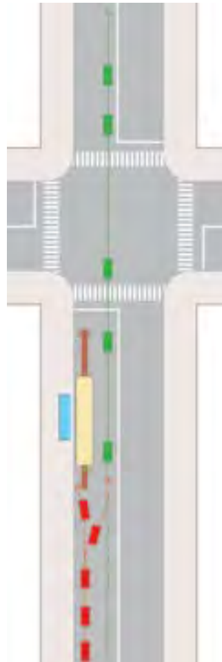
Figure 39. Impact on traffic due to stop positioned before intersection
