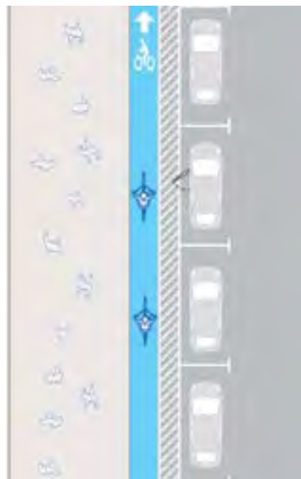
Figure 26. Buffer between cycle lane and parking lane using on-street markings using paint.
