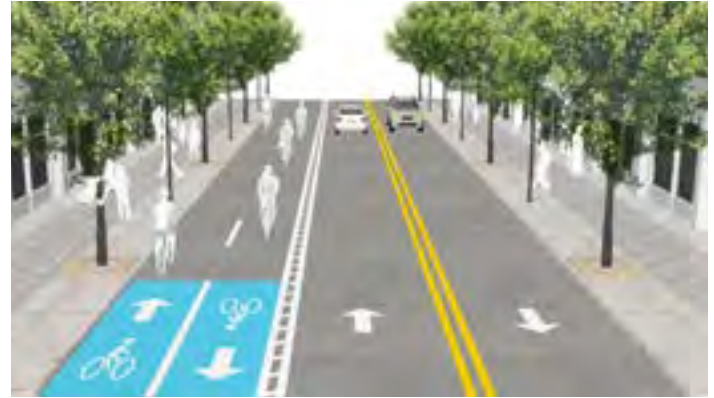
Figure 20. Bi-directional marked cycle lane.
