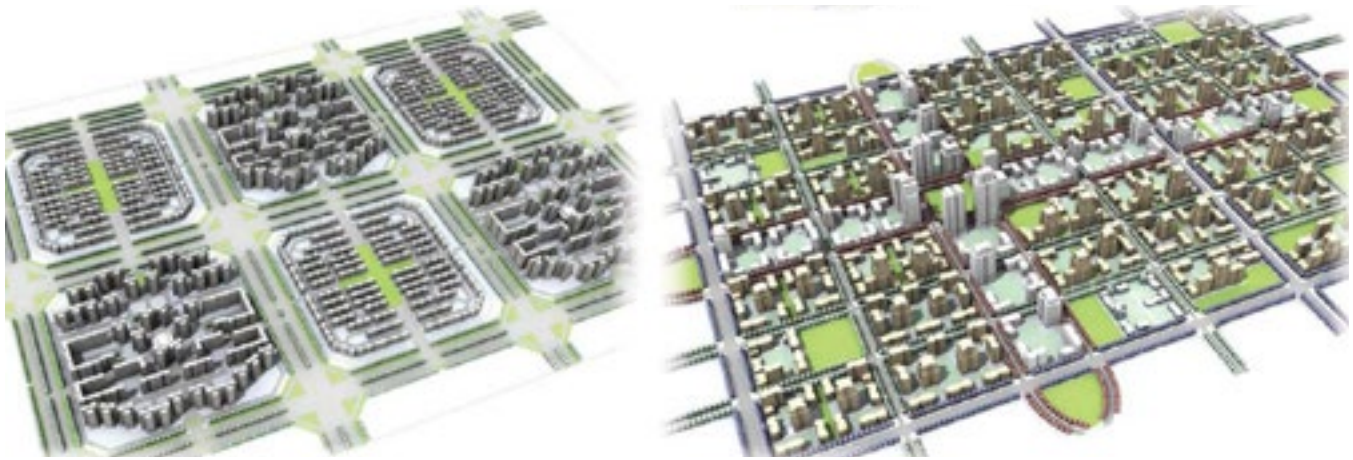
Figure 3-2: Illustrative diagrams depicting the urban form of superblocks (left) and walkable development (right). The diagrams are at the same scale. (Source: HDR | Calthorpe)
