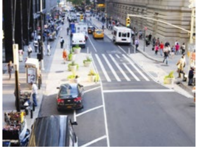
Figure P7-8: Curb extensions (also called bulb-outs) extend the sidewalk into the parking lane or driving lane to provide additional pedestrian space at key locations, usually at corners or mid-block. Curb extensions enhance pedestrian safety by increasing pedestrian visibility, shortening crossing distances, and visually narrowing the roadway. (Source: NACTO)
