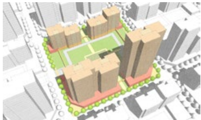
Figure P7-29: Perspective view of a residential block in a shopping street, with a minimum 60 percent of block perimeter dedicated to publicly accessible uses (Source: HDR | Calthorpe)
