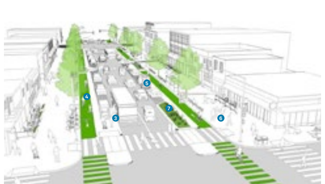
Figure P7-8: Curb extensions (also called bulb-outs) extend the sidewalk into the parking lane or driving lane to provide additional pedestrian space at key locations, usually at corners or mid-block. Curb extensions enhance pedestrian safety by increasing pedestrian visibility, shortening crossing distances, and visually narrowing the roadway. (Source: NACTO)
