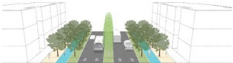
Figure P7-30: Bike lanes should be dedicated and protected on any street wider than four automobile lanes. (Source: Flickr: Rich & Cheryl, CC BY-NC-SA 2.0)
