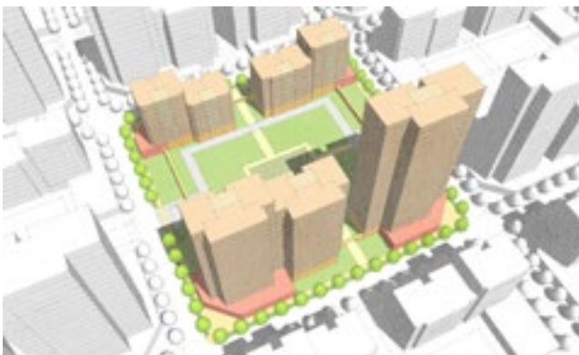
Figure P7-28: Perspective view of a residential block in a non-shopping street, with a minimum 20 percent of block perimeter dedicated to publicly accessible uses (Source: HDR | Calthorpe)
