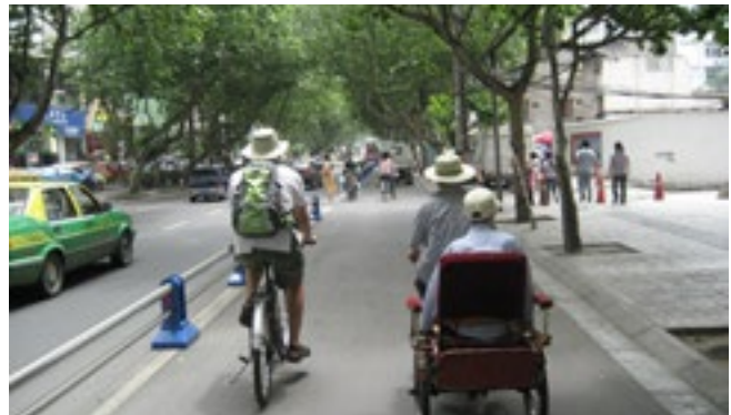
Figure P7-30: Bike lanes should be dedicated and protected on any street wider than four automobile lanes. (Source: Flickr: Rich & Cheryl, CC BY-NC-SA 2.0)
