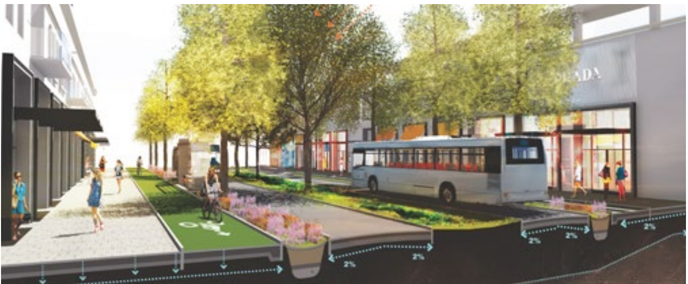
Figure P6-30: A car-free streetscape concept that provides dedicated bike lanes and safe sidewalks, while also allowing dedicated lanes for public transportation. Well-designed landscaping and tree lines enhance the walking and biking experience. (Source: HDR | Calthorpe)
