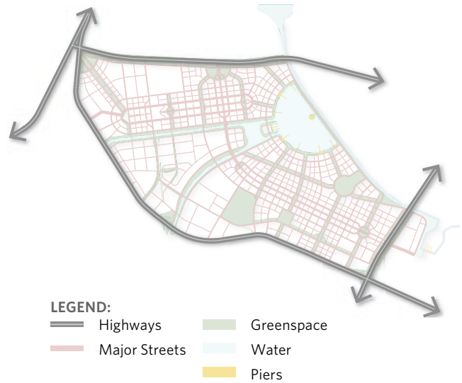
Figure P6-19: This diagram emphasizes the placement of major expressways and highways on the outer edge of the district in North TOD Plan for Zhuhai, China (Source: HDR | Calthorpe)
