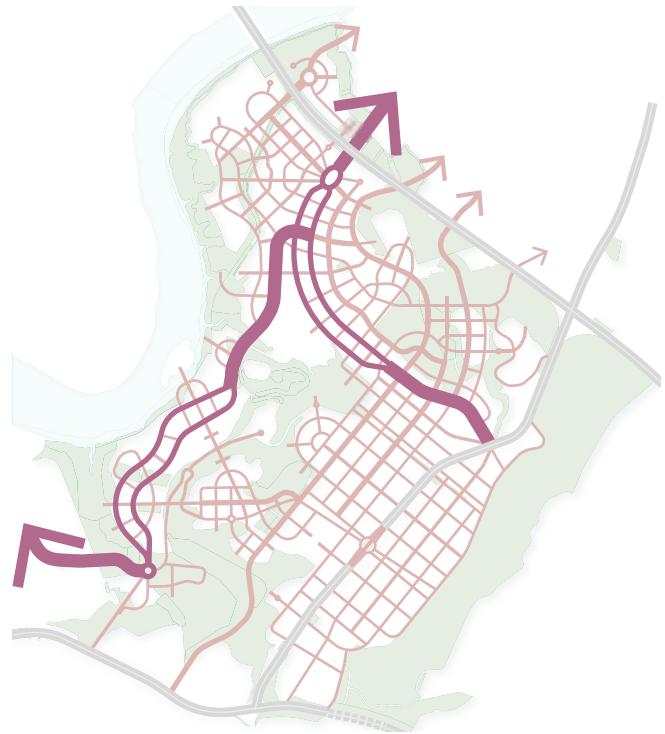
Figure P6-22: Circulation diagram after the introduction of one-way couplet streets within the Yuelai Eco-City, China (Source: HDR | Calthorpe)
