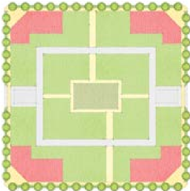
Figure P5-12: An illustration of a 100m x 100m residential block in a non-shopping district showing a minimum 0.15 FAR at block corners (Source: HDR | Calthorpe)
