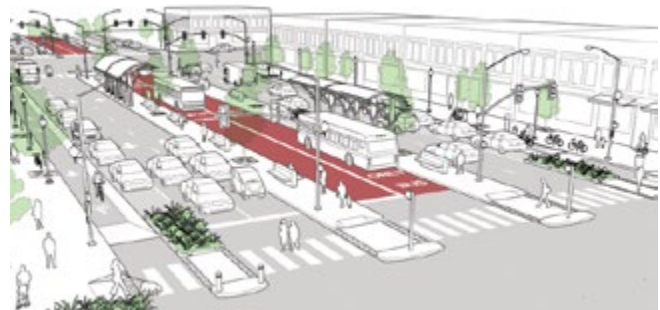
Figure P3-9: Street concept with dedicated bus lanes. Dedicated transit lanes improve transit efficiency, speed, and convenience. (Source: "Urban Street Design Guide," NACTO)
