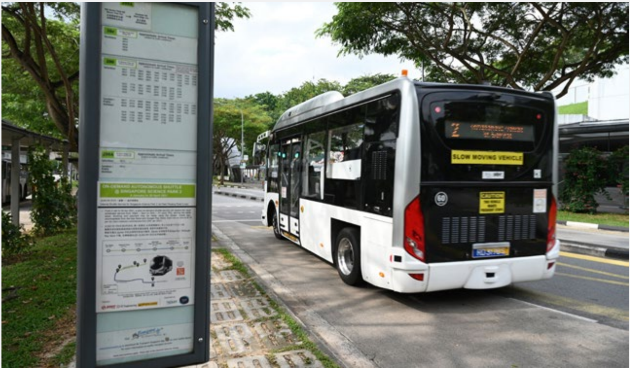
Figure P3-19: An on-demand autonomous bus developed by ST Engineering departs from bus stop after picking up passengers at the start of a trial run from Singapore Science Park 2 to Haw Par Villa MRT station in Singapore on January 26, 2021. (Photo by ROSLAN RAHMAN/AFP via Getty Images)
