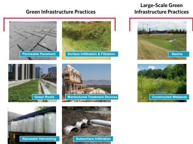
Figure P2-18: Practices for retail/office, residential, and existing industrial land use (Port Authority of New York New Jersey Green Infrastructure Design Manual)
