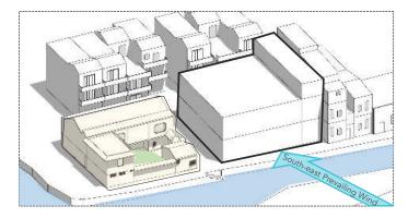
**Reduce the size:** The ground floor and first floor are partially recessed on the western and southern sides to form balconies. This creates a shadow area and a temperature difference within the environment. Moreover, variation in the height of the buildings and the courtyard can facilitate hot pressure ventilation.
