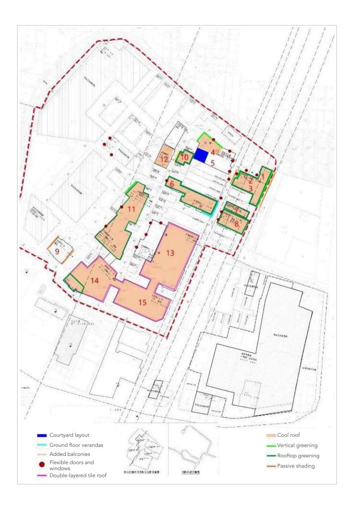
Install a patio inside the building to form a small courtyard, increasing the open interface of the building and improving ventilation.
