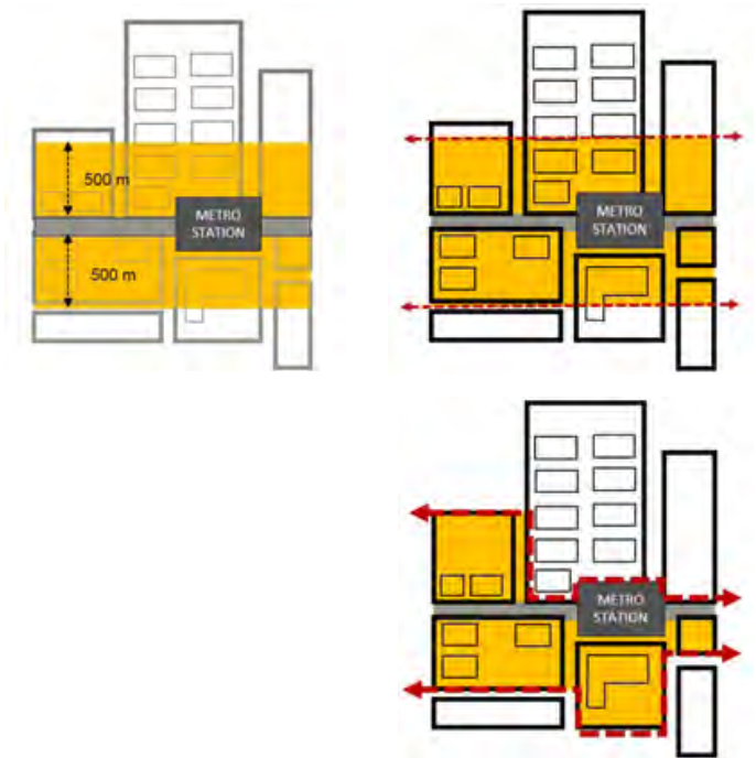
Figure 1: TOD Influence Zone Delineation, Delhi TOD Policy Manual Source: Reproduced from UTTIPEC, WRI India (2014)
