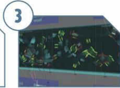
3 ZenRobotics Brain identifies materials, objects and gripping points.
