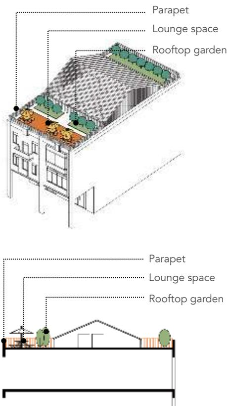
**Figure 24 // INTENSIVE AND EXTENSIVE GREEN ROOF**
