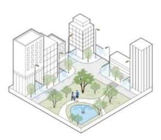
Misting facilities sprinkle very small water droplets at high pressure to lower the surrounding air temperature. Under different climate conditions, misting facilities can reduce the temperature of the surrounding environment by 5 to 15 degrees Celsius. It is common to set up high-pressure misting facilities or fountains in crowded areas.
