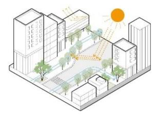
Highly reflective surfaces store and conduct less heat to its interior, in turn helping to reduce building energy consumption and heat waste from air conditioning use. Additionally, with cooler surfaces of the built environment, it can reduce urban ambient temperature and effectively improve human thermal comfort. The benefits of using highly reflective surfaces on urban buildings can be observed on individual buildings, building blocks, entire cities, and even on a global scale.
