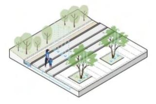
A permeable surface allows rainwater to penetrate into the soil. Water stored in the pavement can absorb a large amount of heat through evaporation and cool the pavement during summer, especially in a dry climate. Therefore, these pervious and porous materials not only improve stormwater management but also facilitate moisture evaporation more efficiently, offsetting the excessive heat released by conventional paved surfaces.
