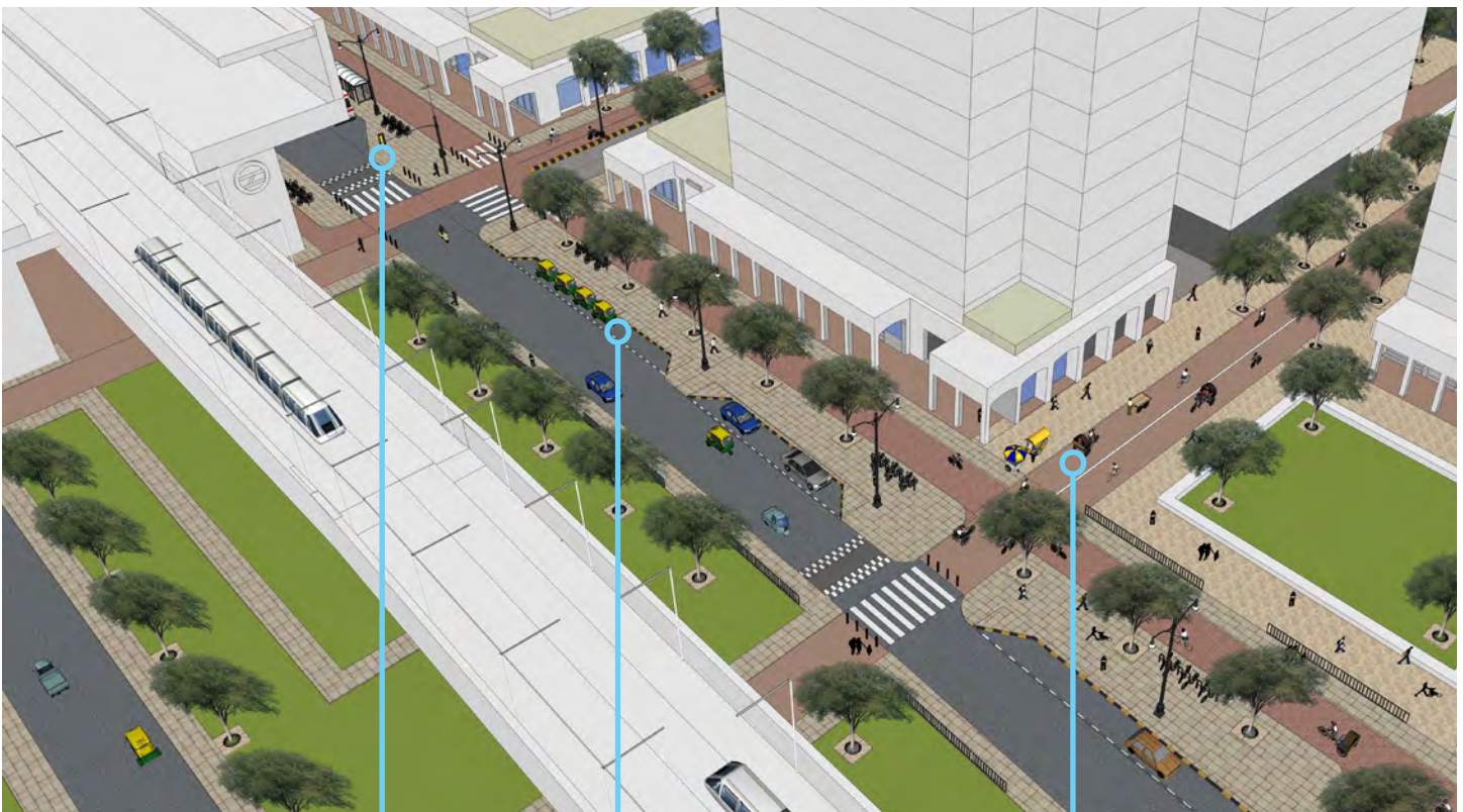
Thane Suburban station in India with lower level for auto-rickshaws and upper levels for bus bays. It connects to the road level via elevated walkways (Source: © WRI India)
