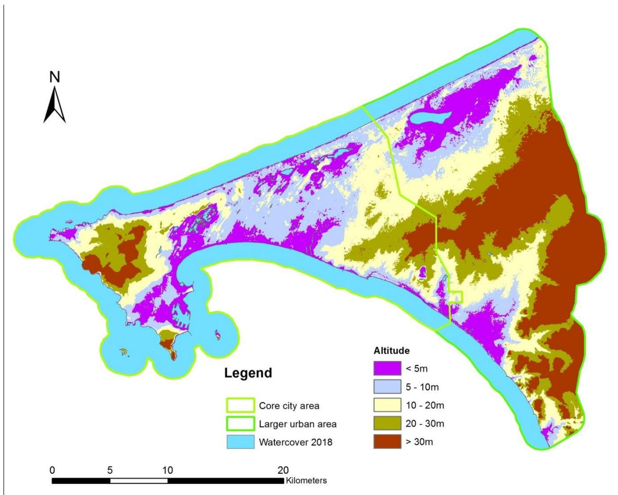
**Figure 31: Altitudes in Dakar Service Area as derived from available Digital Terrain and Surface Models (western part: 5m Digital Terrain Model of Dakar (BaseGéo Sénégal, (<http://www.basegeo.gouv.sn/>) based on Urban Database (UDB) product; eastern part: ALOS Global Digital Surface Model "ALOS World 3D - 30m (AW3D30)", version 2.1 (©JAXA): Amthyst areas indicate most flood prone zones (altitudes below 5 m).**
