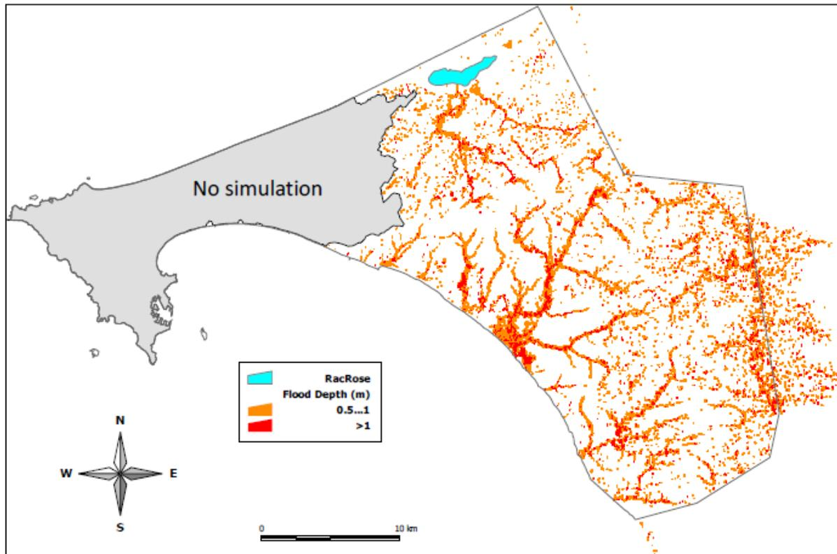
**Figure 34: Possible Flooding Area in the New Urban Expansion Area based on Flo2D modelling results (taken from JICA 2016)**
